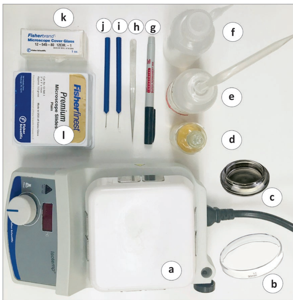
Fig. 6. List of tools needed in rapid slide mounting procedure. (a) Hot Plate, (b) Petri Dish Cover, (c) Watch Glass, (d) Hoyer's Mounting Medium, (e) 10 % Potassium Hydroxide, (f) Distilled Water, (g) Marker, (h) Forceps, (i) Micro-spatula, (j) Micro-scalpel, (k) Microscope Cover Glass 12CIR, and (l) Microscope Slides 3" × 1" × 1 mm (photo credit: M. Z. Ahmed).
